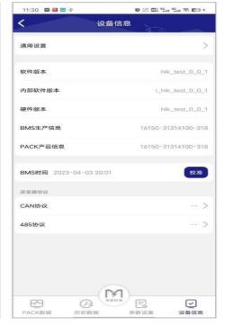
OTA upgrade The original design of the upgrade triggering strategy was for the APP to automatically identify whether an upgrade was needed based on the current software version number of the device. However, due to incorrect responses to MCU software version and other info rmation, it was temporarily triggered by clicking on the device icon.
